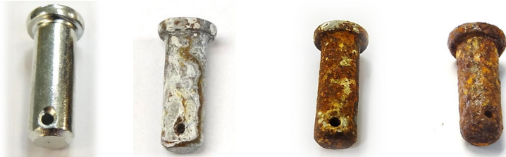
1. New bolt 2. Acceptable 3. Replace 4. NOT acceptable
